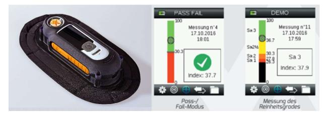
Using a pre-defined reference level of purity or in true / false mode, the device works reliably and you can document and archive the collected data without software in Excel.
